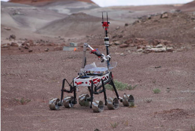
Fig. 15 Team R3's rover being teleoperated by the simple_drive ROS package
