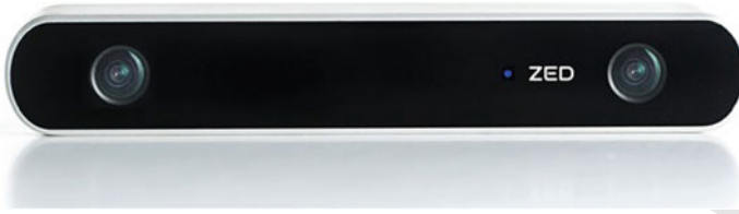
Fig. 24 The ZED depth camera. Image credit: Stereolabs
